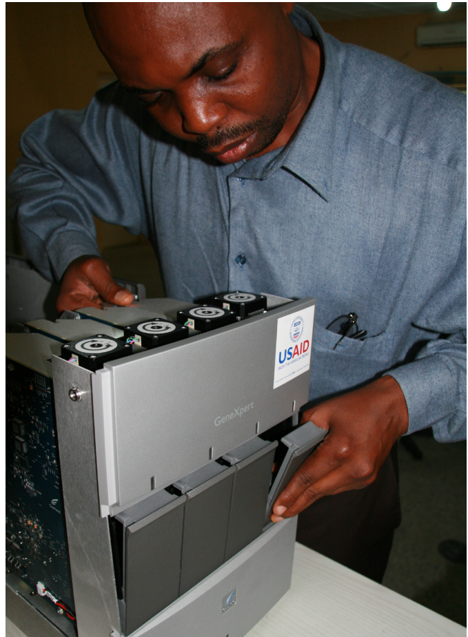
Laboratory supervisor preparing GeneXpert instrument for annual calibration, Nigeria
